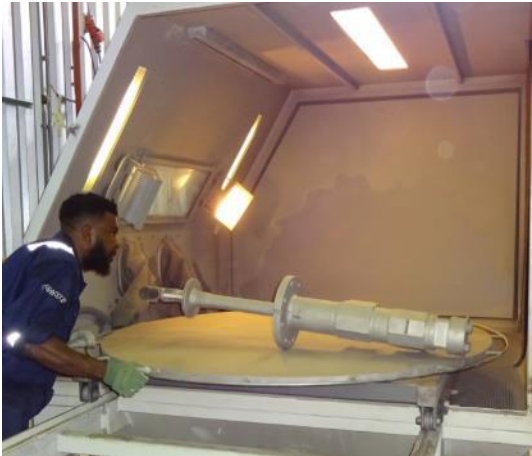
Grit Blasting / Cleaning
